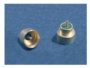
The SMP snap-on connector has become a popular RF connector for use in high density RF system packaging.
